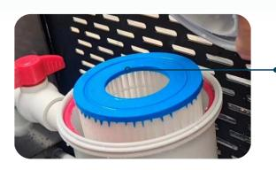
When replacing the filter element, please close the water inlet and outlet valves of the tub, loosen the filter exhaust valve by counter clockwise, then unscrew the filter cover, remove the filter element, and replace the filter element.
