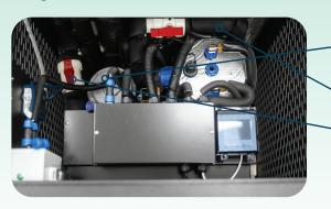
Open the hatch on the top and you can change the filter and open/ close ball valves inside.
