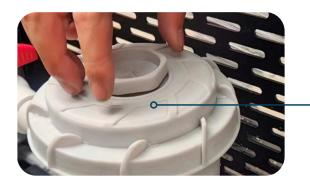
After replacing the filter element. Screw on the filter cover, open the ball valves. Then open the exhaust valve slightly to ensure there are no air locks. After this you can turn the Ice bath back on
