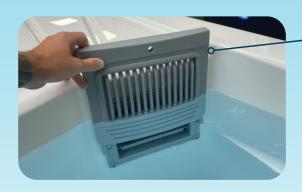
Now the filter housing can be removed. To remove the filter housing, pull the housing vertical and slide up.
